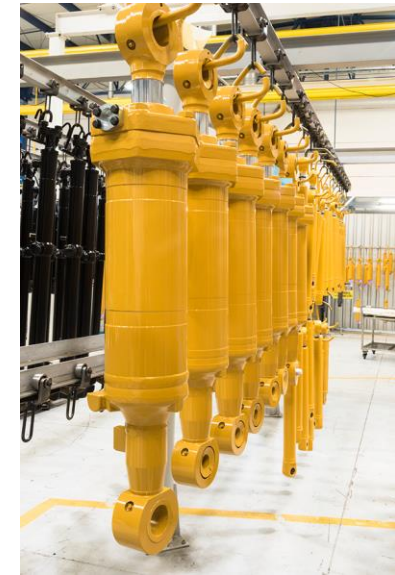
Hidrover – “Double action” cylinders
